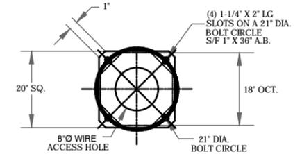
**SPUNCAST, PRESTRESSED CONCRETE POLE**
