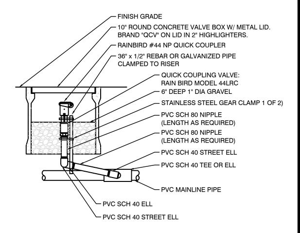
NOTE: FURNISH FITTINGS AND PIPING NOMINALLY SIZED IDENTICAL TO NOMINAL QUICK COUPLING VALVE INLET SIZE.
